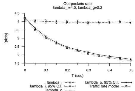
Figure 8. Out-packet ( $\lambda_{out}$ ) and in-packet ( $\lambda_{in}$ ) rates, for different values of  $T$ , and a theoretical in-packet rate  $\lambda_{in} = 4\frac{pkts}{s}$  (simulations and analytical results).
