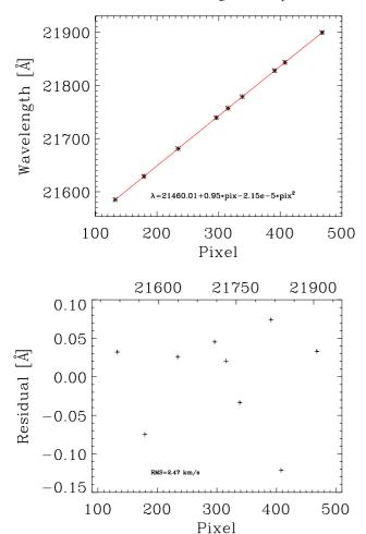
**Fig. B.2.** *Top*: calibration between the pixel and wavelength values of the VLTI/AMBER observations of MWC 297. A least-square polynomial fit of the data is also shown (red line). *Bottom*: residuals between the measured position of the telluric line spectrum obtained from the wavelength calibration of the AMBER data and the expected position from the reference telluric spectrum provided by NOAO. The root-mean square value is of the order of 2.5 km s<sup>-1</sup>.
