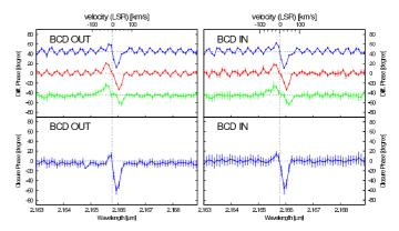
**Fig. C.1.** Differential phases and closure phases derived from the data obtained without (*left*, BCD OUT) and with (*right*, BCD IN) the beam commutation device. The shown signals are not yet corrected using the calibrator data. After we corrected the sign changes introduced by the BCD device, the two data sets yield the shown signals, which are nearly identical and demonstrate the high accuracy of the measured phase signals.
