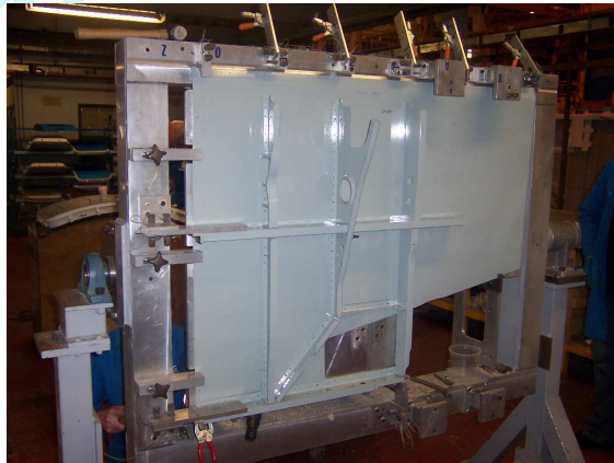
Fig. 14 Uplock and Apron Assembly (With Fixture)
