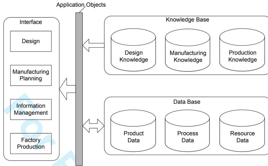
Fig.1 Architecture for a modern digital manufacturing system
