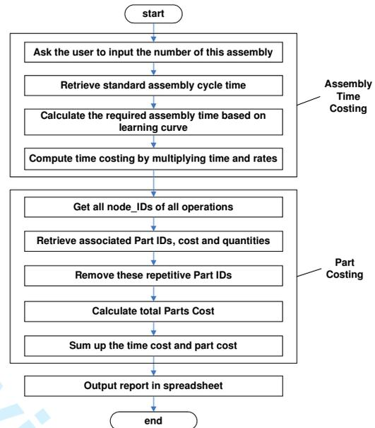
Fig. 13 Flowchart for calculating assembly cost
