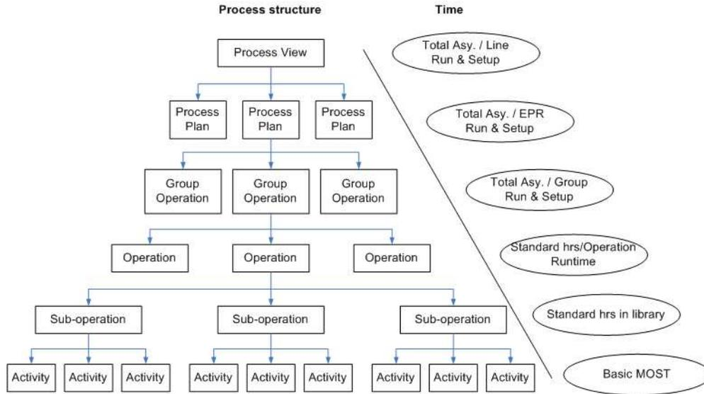
Architecture of work breakdown structure utilized in time analysis
