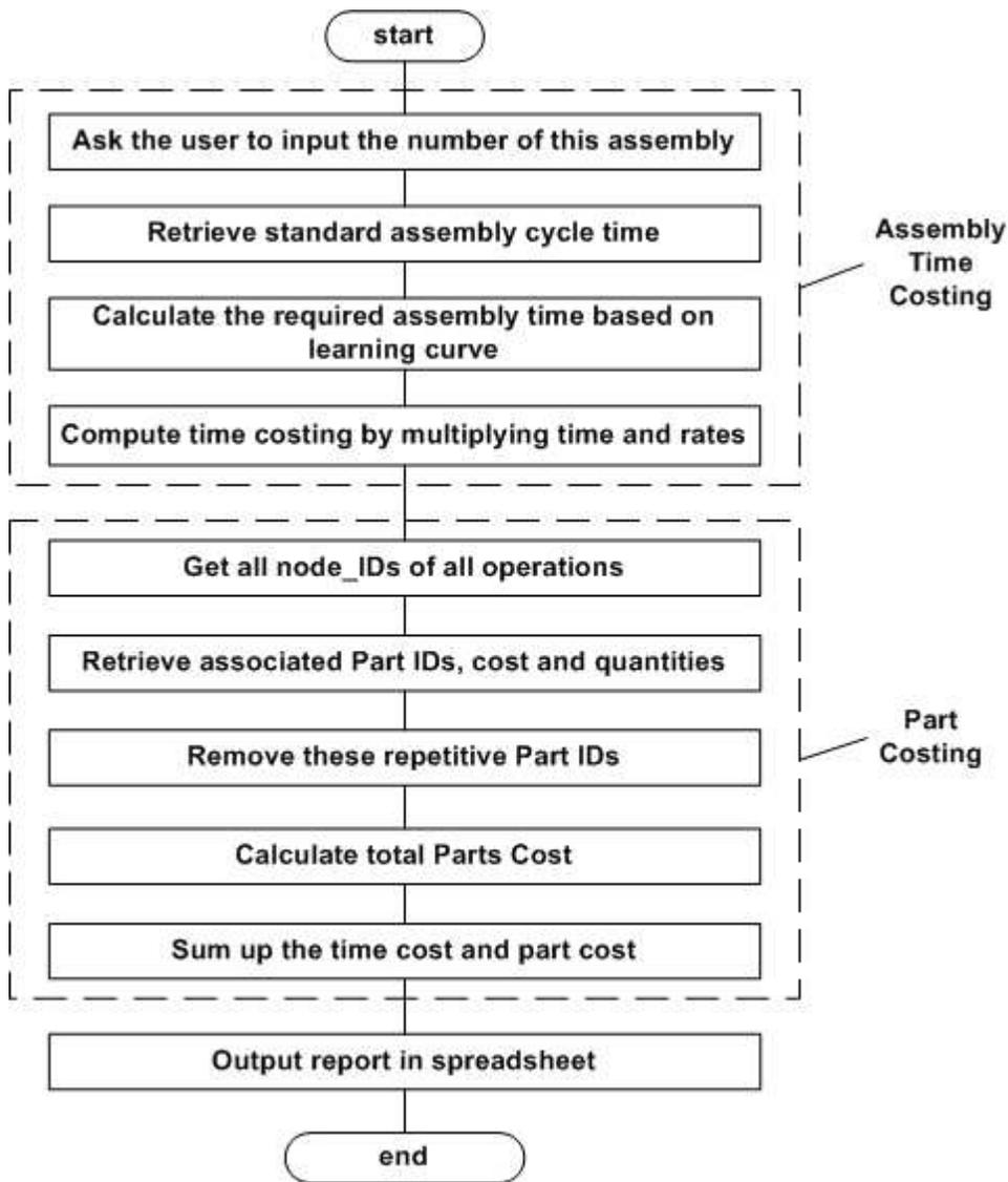
Flowchart for calculating assembly cost
