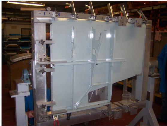
Fig. 14 Uplock and Apron Assembly (With Fixture)
