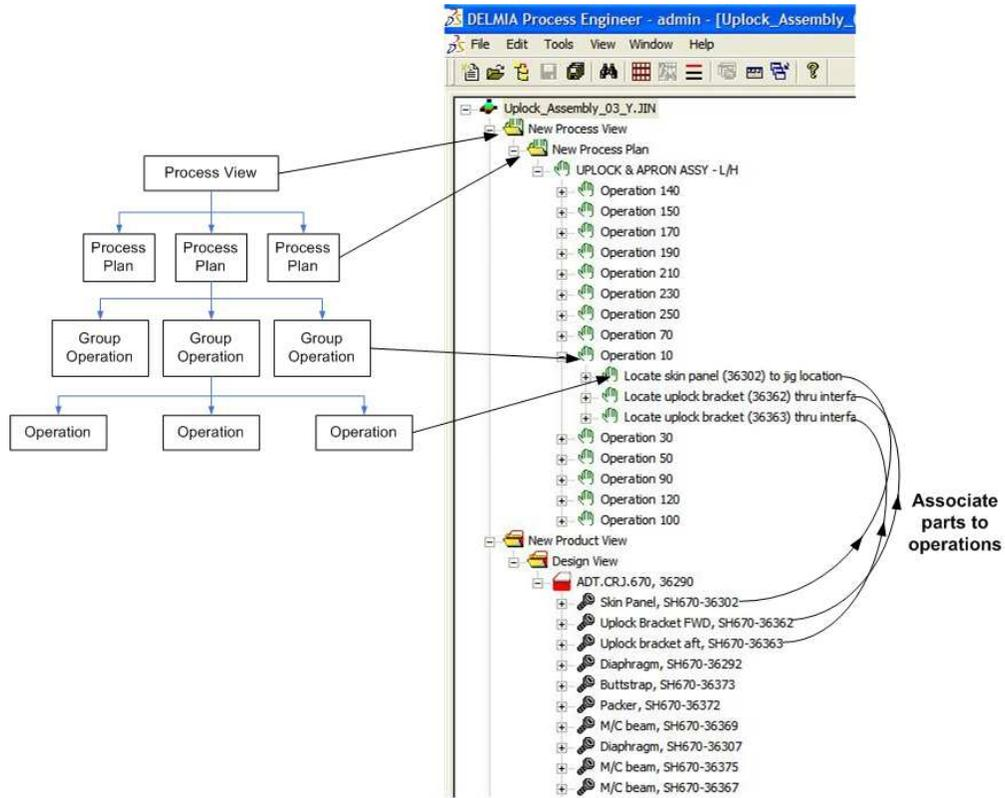
Implementation of the object oriented process structure in DPE
