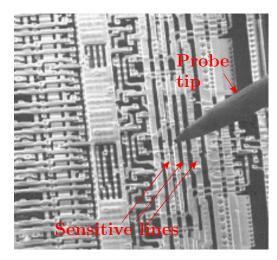
Figure 1. Probing of a circuit thanks to prober tip, to read or force sensitive variables (courtesy of [4], Fig. 4.1 of §4.2. at page 31).
