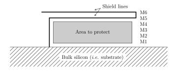
Figure 3. General structure of a shield (sagittal view).
