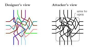
Figure 7. The figure on the *left* illustrates the *N* segments making up an active random shield. The connectivity of these segments (indicated with N = 8 different colors) is unknown to the attacker; the figure on the *right* shows the vision of an attacker who discovers the shield.
