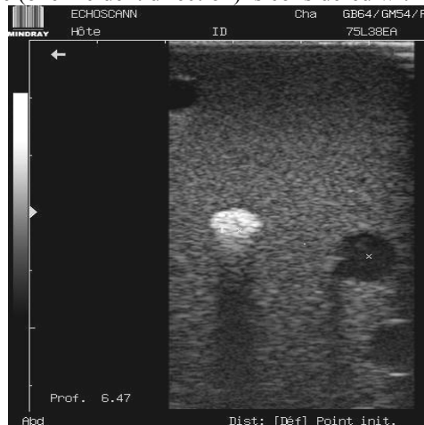
Figure 3: Echographic view (Mindray, 7.5 MHz) of breast training phantom CIRS Model 052A
