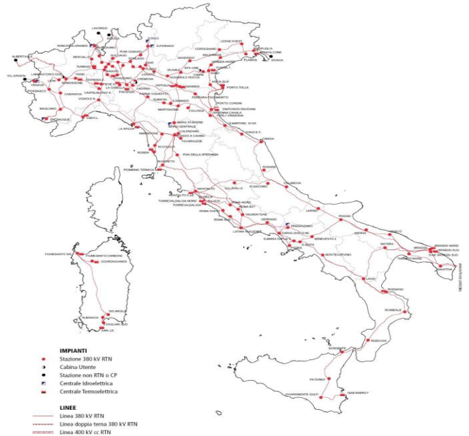
Figure 1. The 380 kV Italian power transmission network [TERNA 2002, Rosato et al. 2007].
