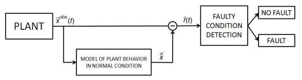
Figure 1. Condition monitoring scheme
