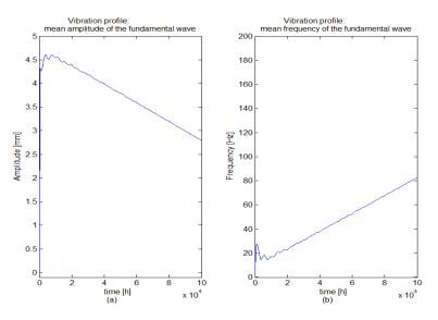
**Figure 5:** vibration profile applied to the component, in terms of mean amplitude (to the left) and mean frequency (to the right).
