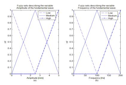
Figure 4: fuzzy sets of the variables in input to the Backward Module.
