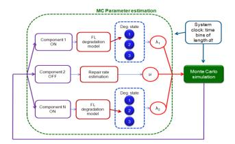
Figure 2: interface between FL degradation models and MC simulation.
