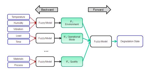
Figure 1: snapshot of the FL degradation model.
