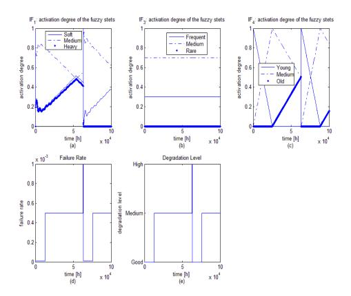
**Figure 8:** activation degree of the IFs fuzzy sets and of the degradation state, failure rate value and defuzzyfied degradation state considering a control period of 7000 *h* when no failure occurs.
