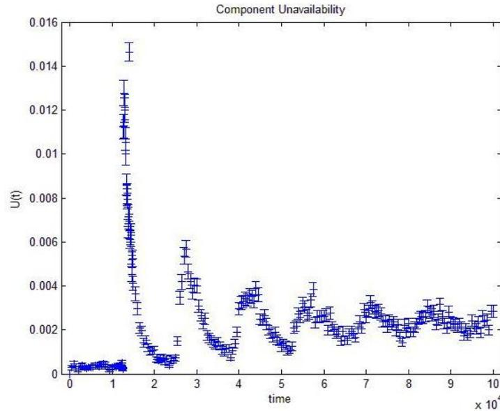
**Figure 9:** instantaneous component unavailability and its standard deviation.
