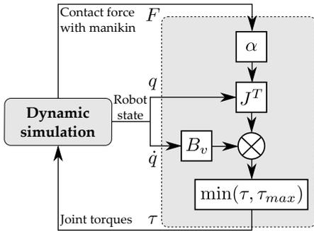
**Figure 3.** Block diagram of the robot control framework.
