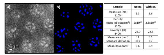
**Figure 2.** EFTEM image of a ULE-IBS prepared sample through the BC a) plan-view, b) binarisation of image a) for image analysis, c) Characteristics of the Ncs population deduced from the image analysis. Roundness =  $4Pi^*$ Area/Perimeter<sup>2</sup>.
