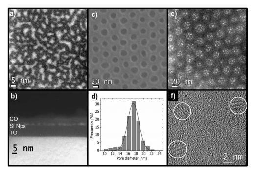
**Figure 1.** EFTEM images of ULE-IBS prepared samples without BC mask a) plan-view and b) cross-section and through the BC mask e) plan-view. c) SEM image of the BC mask and d) the corresponding pore diameter distribution. f) HRTEM image of crystalline nanoparticles.
