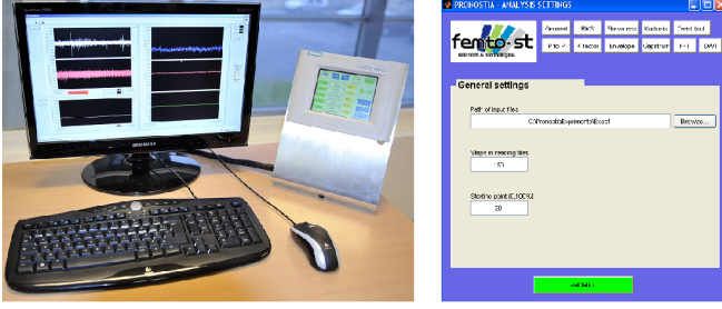
Fig. 4. (left) Labview VI for raw signal visualization and (right) the graphical user interface to set the optional parameters (if required) of the signal processing algorithms.
