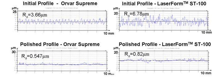
Figure 7: Initial and final roughness profiles for Orvar Supreme (left) and LaserForm<sup>TM</sup> ST-100 (right)
