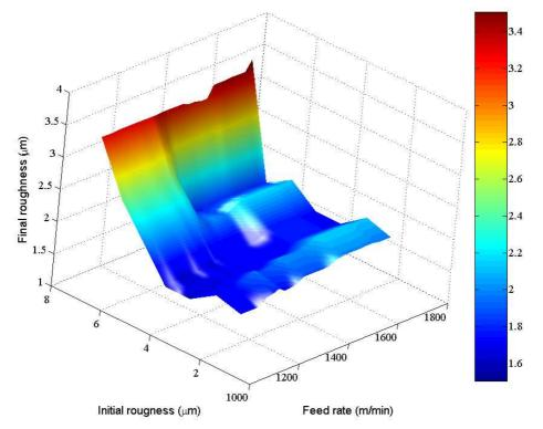
Figure 12. 3D Plot of industrial interest: final roughness as a function of feed rate and initial roughness.
