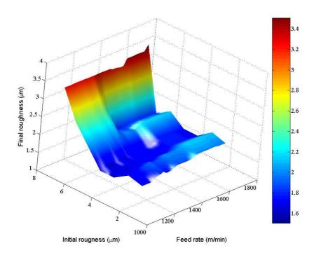
Figure 12. 3D Plot of industrial interest: final roughness as a function of feed rate and initial roughness.
