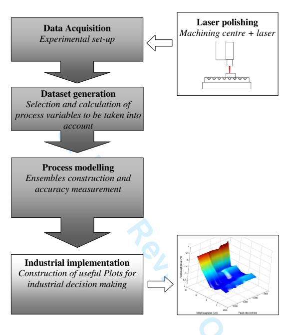
Figure 1. Scheme of the soft computing tool for surface roughness prediction.
