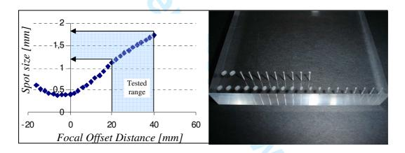
Figure 3. Relationship between spot size and focal offset distance for a fixed laser power
