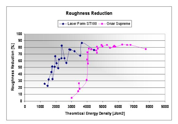
Figure 8. Measured roughness reduction for different theoretical energy densities in LaserForm<sup>™</sup> ST-100 and Orvar Supreme steel
