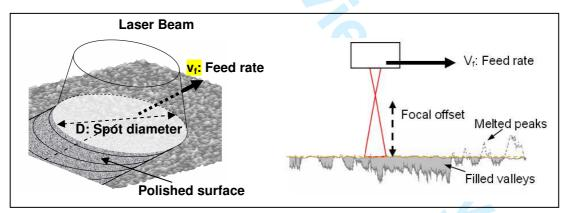
Figure 2. Laser polishing scheme
