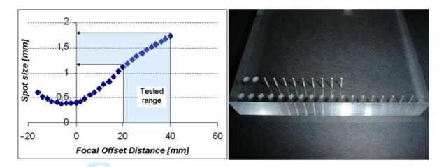
Figure 3. Relationship between spot size and focal offset distance for a fixed laser power
