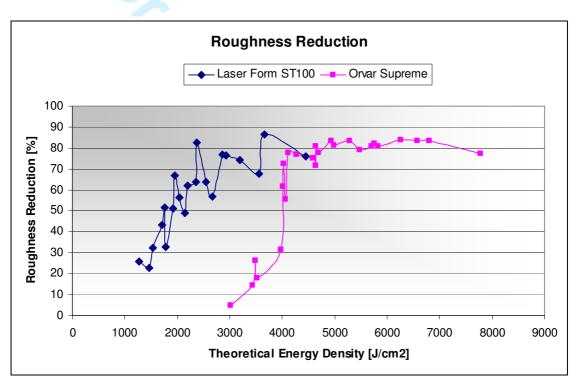
Figure 8. Measured roughness reduction for different theoretical energy densities in LaserForm<sup>™</sup> ST-100 and Orvar Supreme steel
