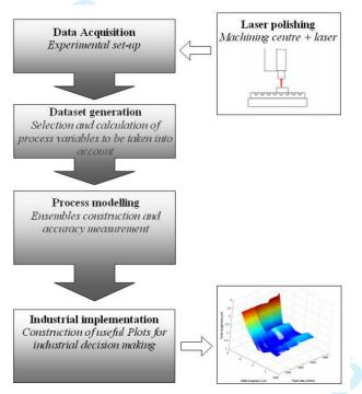
Figure 1. Scheme of the soft computing tool for surface roughness prediction.
