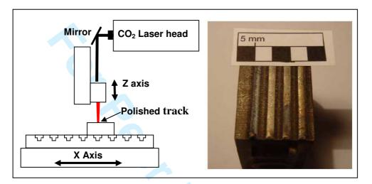
Figure 4: Experimental set-up for the laser polishing test and laser polishing test parts of LaserForm<sup>TM</sup> ST-100
