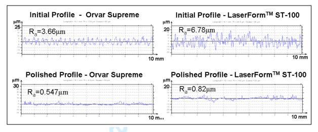
Figure 7: Initial and final roughness profiles for Orvar Supreme (left) and LaserForm<sup>TM</sup> ST-100 (right)
