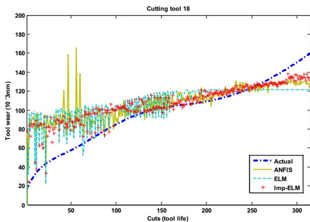
Fig. 7. Tool wear predictions for a multi-tools model - poor reliability illustration on an unknown cutter
