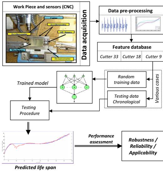
Fig. 4. Methodology for cutting tool wear prediction
