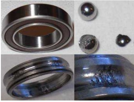
Fig. 6. Normal and degraded bearing.
