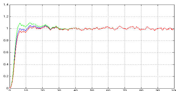
Fig. 11 Output power responses for wind speeds equal to 12m/s (red), 18m/s (blue) and 25m/s (green)
