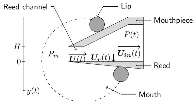
Figure 1: Schematic diagram of a single-reed mouthpiece. Presentation of variables, control parameters and choice of axis orientation.  $U$  is the flow created by the pressure imbalance  $P_m - P$  between the mouth and the bore,  $U_r$  is the flow created by the motion of the reed,  $U_{in}$  is the flow entering the instrument,  $y$  represents the position of the tip of the reed and  $H$  is the opening of the reed channel at rest.
