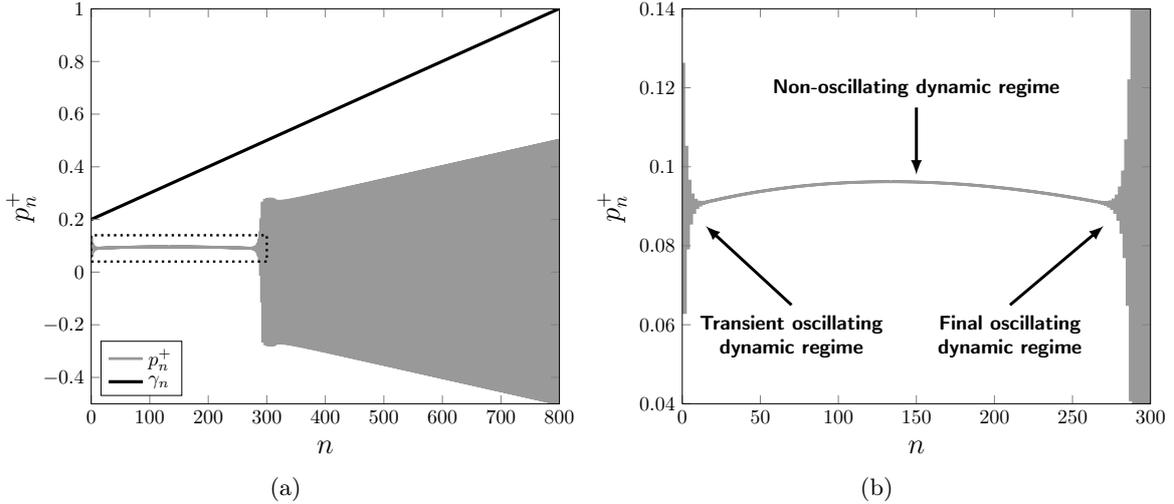
Figure 4: Numerical simulation performed on the system (23). (a) complete orbit of the series and (b) zoom near the non-oscillation dynamic regime.  $\zeta = 0.5$ ,  $\epsilon = 10^{-3}$ ,  $\gamma_0 = 0.2$  and  $p_0^+ = G(0, \gamma_0)$ .
