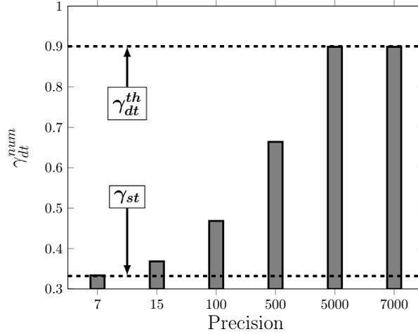
Figure 9: Graphical representation of  $\gamma_{dt}^{num}$  for different precisions (prec. = 7, 15, 100, 500 and 5000) and for  $\epsilon = 10^{-4}$ . Results are also compared to analytical *static* and *dynamic* thresholds:  $\gamma_{st}$  and  $\gamma_{dt}^{th}$ .  $\zeta = 0.5$  and  $\gamma_0 = 0$ .
