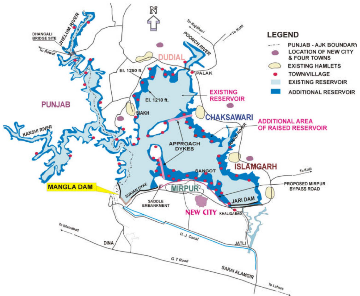
Fig. 1 Layout of Mangla dam extension works, affected towns, and location of resettlement sites. (Image courtesy: WAPDA)
