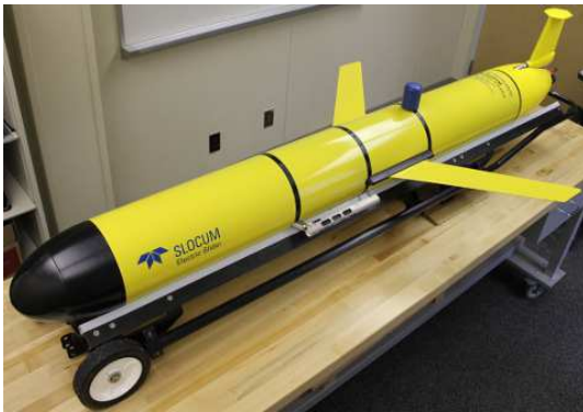
Fig. 1. One of our Slocum glider autonomous underwater vehicles equipped with a double payload bay and an acoustic modem. The shown configuration is 180 cm long and weighs about 90 kg.
