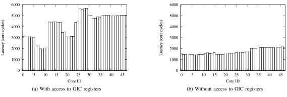
Fig. 2: Latency of broadcasting an interrupt at the kernel level
