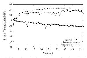
Fig. 3: Throughput of the asynchronous broadcast algorithm for different values of k and different number of concurrent sources
