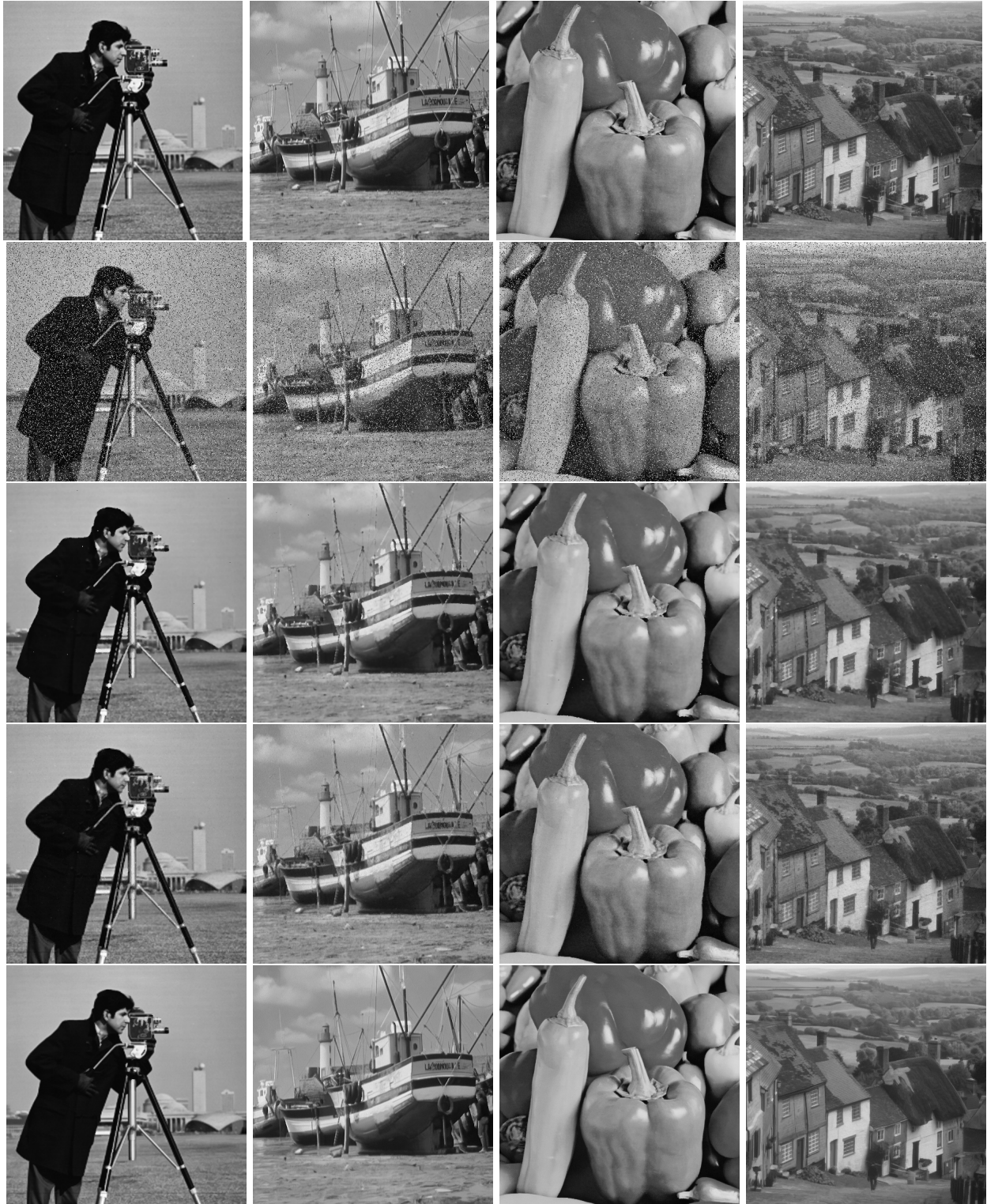
FIG. 6.3. Comparative results on Cameraman, Boat, Peppers and Goldhill with p = 20\% of random-valued impulse noise. For each column, from top to bottom: original image, noisy image, ROAD+trilateral [25], ROLD+EPR [21], PARIGI. Images should be seen at full resolution on the electronic version of the paper.
