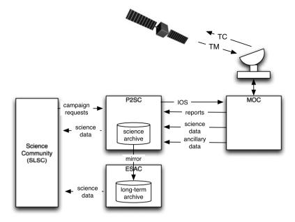
Figure 1 The PROBA2 ground and flight segments.
