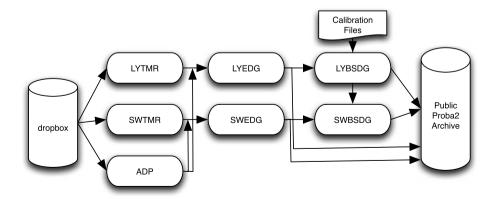
Figure 2 Architectural overview of the P2SC data processing.
