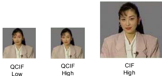
Fig. 11. Quality-Spatial six-layered test sequence structure. – temporal resolution omitted.
