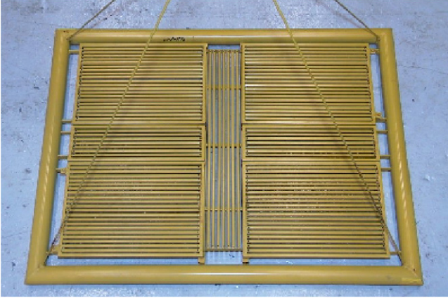
Fig. 2. Example of ventilated structure, a protection cover for subsea modules [1].
