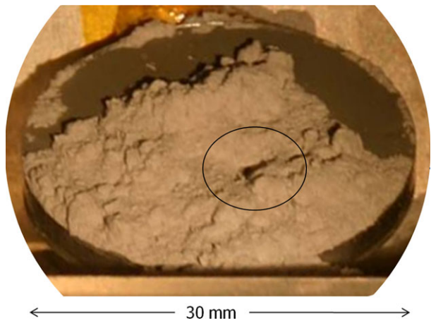
Fig. 26 Test of LIBS profile through thick dust. Loose dolomite dust was placed on a pressed basalt target, lying at an \sim 45^\circ angle. Circle indicates the pit created by the laser pulses
