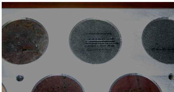
Fig. 13 Engineering model shergottite calibration target ( center of image ) after 15,000 laser pulses as part of the sample consumption test
