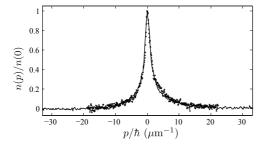
FIG. 4: Momentum distribution of a gas of about 7000 atoms at thermal equilibrium, in a 7.5 Hz longitudinal trap, and 4.6 kHz transverse trap. The solid distribution is obtained without levitation and with a free fall of 24.7 ms. The circles are the momentum distribution of the same sample, but with a levitation time of 20.6 ms followed by a free fall of 22.7 ms.
