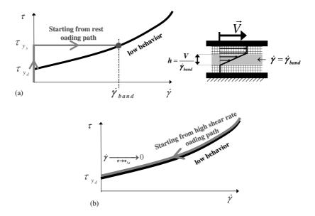
Figure 4: Illustration of the procedure-dependent behavior in a material whose static and dynamic yield stresses differ: (a) a band may form at flow start-up (Sec. 2.3.1); (b) an initially homogeneous flow may remain stable and homogeneous at any rate when the applied shear rate is decreased (Sec. 2.3.2).
