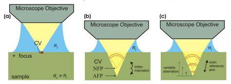
Fig. 2. Principle of the method used to create known aberration. (a) Initial state at the surface of the sample (no aberration). (b) When focusing into the sample, the index mismatch moves the CV and the AFP in opposite directions away from the NFP and introduces tractable aberrations. (c) By changing the reference arm length, the CV position can be further displaced to add or subtract aberrations.
