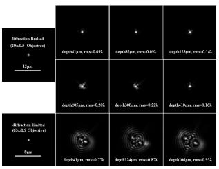
Fig. 7: Point Spread Function as extracted from the wavefront measured by CGWS for the minimal defocus position using the first 28 coefficients. The PSF was scaled over the whole gray values (0-255). We observe that the PSF degrades notably over the range of reliability of the CGWS.
