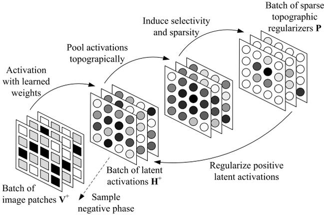
**Fig. 1.** The framework for inducing both sparseness and topographical organization. From a batch of pixel inputs  $\mathbf{V}^+$ , the latent units are activated  $\mathbf{H}^+$  via learned weights. The activations are then topographically pooled based on the locality of  $h_j$  in the feature map via fixed weights. Subsequently, population and lifetime sparseness are induced to obtain  $\mathbf{P}$ . Finally,  $\mathbf{P}$  is used to regularize the learning of the parameters.
