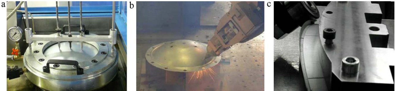
Fig. 5. (a) Biaxial expansion giving the sample curved surface, (b) laser trimming and (c) roll hemming set up.
