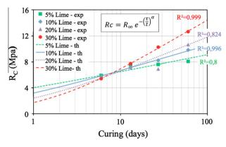
**Fig. 9.** Pumice-lime binders compressive strength evolution with lime mass content and time.
