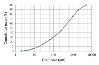
Fig. 2. Pumice sand granulometric curve.
