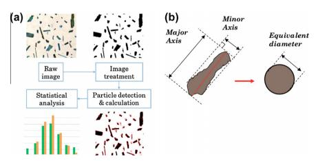
Fig. 4. Vegetable aggregate image treatment procedure (a) and particle size parameters determined with ImageTool software calculation (b).
