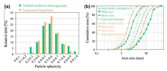
Fig. 5. Granulometry analysis of hemp and sunflower stem aggregates samples made by image treatment method. Aggregates relative area distribution for several particle sphericity classes (a) and cumulative area distribution of previously defined particle size parameters (b).
