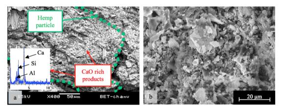
Fig. 13. Hemp hurd particle surface coating (a) and CaO rich phases (b). SEM observations made on H-5 MPa mix.
