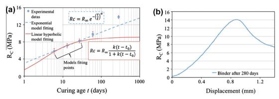
**Fig. 10.** Compressive strength evolution during curing and comparison between linear hyperbolic and exponential models (a), mechanical behaviour at 280 days compressive test (b) for the pumice-lime binder B-5 MPa.
