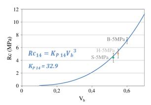
**Fig. 15.** Binder and elaborated plant concrete compressive strength at 14 days as a function of binder solid volume  $V_b$ . Comparison with Powers law model for binder compressive strength (solid curve).
