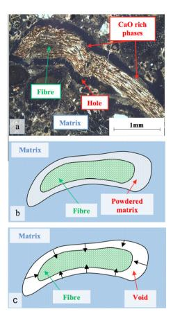
**Fig. 14.** H-5 MPa mix matrix-plant particle interface observation in optical microscopy (a), hypotheses concerning matrix/fibre interface: particle surrounded by powdered matrix (b), and particle surrounded by void (c).
