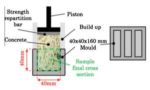
Fig. 3. Concrete mixture compaction process.
