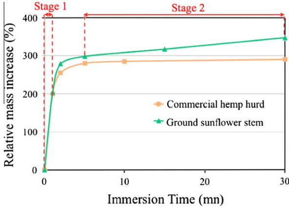
Fig. 8. Mass relative water absorption of commercial hemp hurd and ground sunflower stem aggregate.
