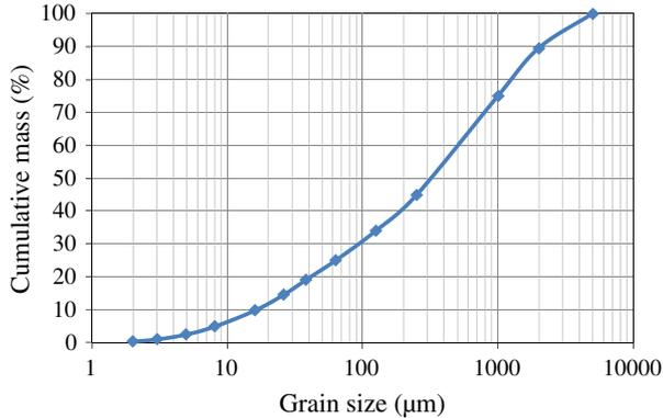
**Fig. 2.** Pumice sand granulometric curve.
