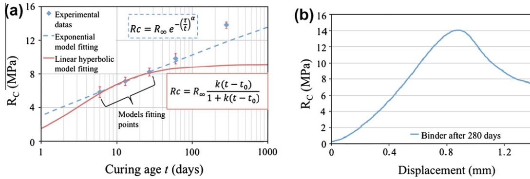
**Fig. 10.** Compressive strength evolution during curing and comparison between linear hyperbolic and exponential models (a), mechanical behaviour at 280 days compressive test (b) for the pumice–lime binder B-5 MPa.
