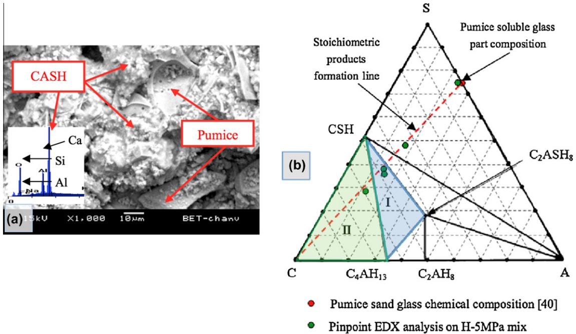
Fig. 12. H-5 MPa matrix SEM observation (a) and resulting EDX analysis carried forward in a CaO–Al<sub>2</sub>O<sub>3</sub>–SiO<sub>2</sub>–H<sub>2</sub>O ternary phase diagram (b).
