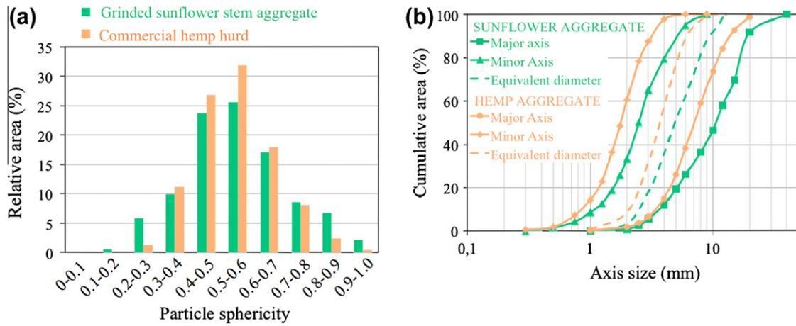
**Fig. 5.** Granulometry analysis of hemp and sunflower stem aggregates samples made by image treatment method. Aggregates relative area distribution for several particle sphericity classes (a) and cumulative area distribution of previously defined particle size parameters (b).
