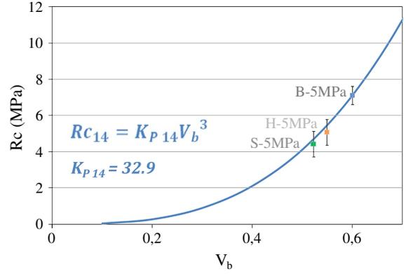
**Fig. 15.** Binder and elaborated plant concrete compressive strength at 14 days as a function of binder solid volume  $V_b$ . Comparison with Powers law model for binder compressive strength (solid curve).
