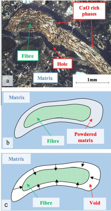
**Fig. 14.** H-5 MPa mix matrix-plant particle interface observation in optical microscopy (a), hypotheses concerning matrix/fibre interface: particle surrounded by powdered matrix (b), and particle surrounded by void (c).
