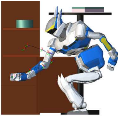
Fig. 1: Goal config generated on the goal submanifold \mathcal{M}_g and a path found by the constrained path planner in a shelves environment.
