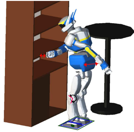
Fig. 3: Constraints added in OCP: support foot positions (blue), joint limits (purple), ZMP constraint (green), (self-)collision avoidance (red).
