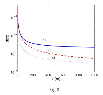
Figure 8 shows the dependence of the precision of our measurements on the distance z (curve a of Fig. 8). An accuracy of  $10^{-6}$  is achieved for long distances z > 50 m. At short distances, the accuracy is dominated by the measurement of  $v_{RT}$  and  $v_{RF}$ . At long distances, it is
