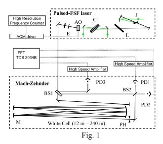
The set-up is depicted in Figure 1. The pulsed-FSF laser is detailed in reference [8]. Briefly, the laser cavity consists of two dye amplifier media. The dye-jet (J) is pumped by a cw
