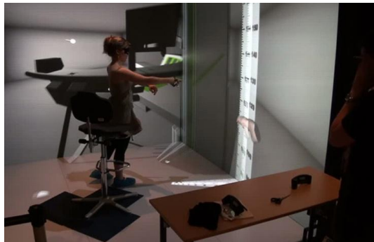
Figure 6. Advanced ergonomic-style convergence support tool (moving around the virtual model, graspable height gauge)
