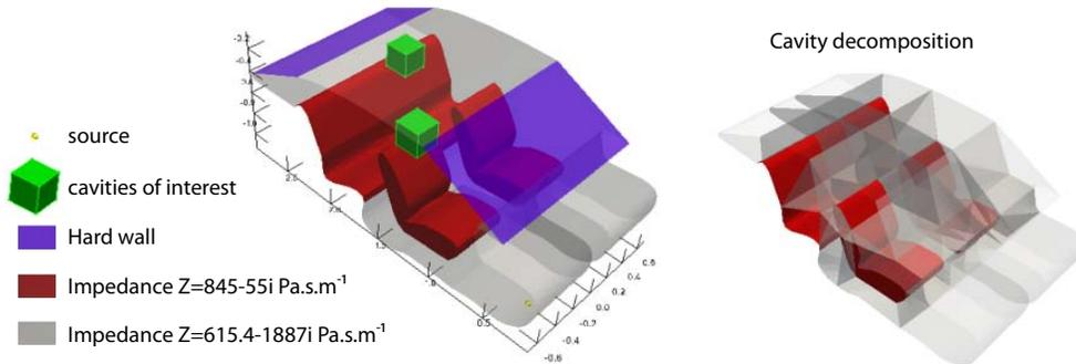
Figure 12. Definition of the car cavity of section 4.3 (boundary conditions on the left and decomposition into sub-cavities on the right).
