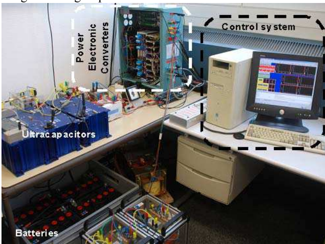
Fig. 18. Prototype hybrid system for the experimental test.
