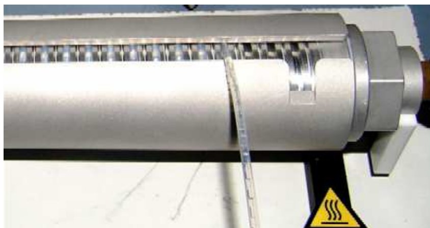
Figure 13. Picture of the main part of the droplet-based millifluidic device used at the laboratory.
