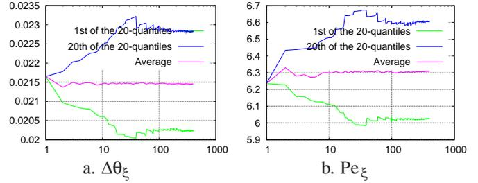
Figure 1. CONVERGENCE FOR THE ELEMENTARY APPROACH OF  $\langle \widehat{X}_\xi \rangle^{[i]}$ ,  $\widehat{V}_1^{[i]}$ , AND  $\widehat{V}_{20}^{[i]}$  AS A FUNCTION OF THE NUMBER OF MONTE CARLO RUNS ( $i$ ) FOR a.  $\Delta\theta_\xi$  AND b.  $Pe_\xi$ .
