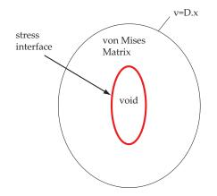
Fig. 1. Schematic diagram showing the hollow spheroid with a stress interface.
