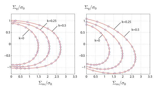
Fig. 4. Yield loci for an oblate cavity with an aspect ratio  $a_1/b_1 = 1/2$  (at the left)  $a_1/b_1 = 1/5$  (at the right) and a porosity f = 0.1.
