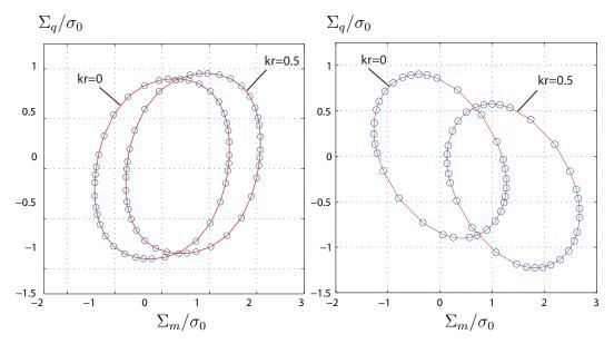
Fig. 5. Yield loci for a prolate cavity with an aspect ratio  $a_1/b_1 = 5$  (at the left) for an oblate cavity with  $a_1/b_1 = 1/5$  (at the right) and a porosity f = 0.1 and for two values of the parameter  $k_r = \tau_r/(b_1\sigma_0)$ .
