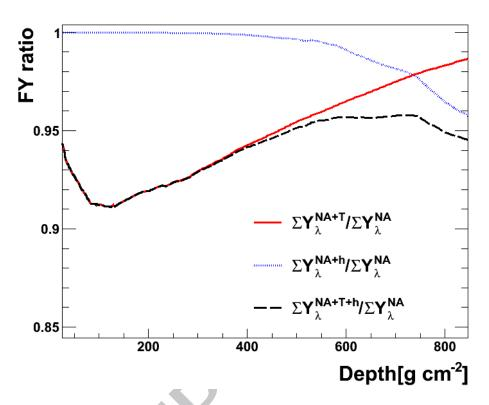
Figure 3: Effect of the humidity and a T-dependent collisional cross section on the N-A data set. In this plot the ratio of fluorescence yields for the month of December versus atmospheric depth is shown.
