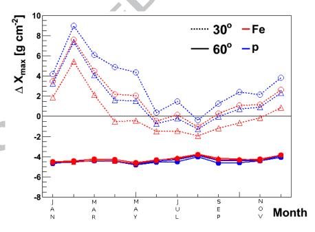
Figure 8: Increase of shower maximum depth due to humidity and a collisional cross section dependent on temperature to the N-A data set, versus month. See figure 7 for more details.
