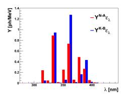
Figure 2: Fluorescence yield in absolute units versus wavelength for the N-A and K-B data sets (left). Since K-B intensities are given in 9 nm bins [9], the N-A fluorescence yields have been recalculated for the same wavelength bins for a better comparison. The effect of the Auger optical efficiency (black line) on the FY of both data sets is illustrated (right).
