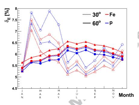
Figure 7: Percentage increase in reconstructed  $E_0$  value when including humidity and a collisional cross section dependent on temperature to the N-A data set, versus month. Results are shown for both protons and Fe nuclei of  $10^{19}$  eV (triangles) and  $10^{20}$  eV (circles) energies.
