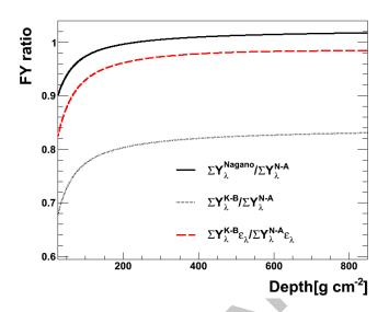
Figure 1: Ratio of Nagano and Kakimoto-Bunner fluorescence yields to that of Nagano-AIRFLY versus atmospheric depth. The ratio K-B/N-A of  $\Sigma Y_{\lambda}(X)\varepsilon_{\lambda}$ , also displayed, indicates that the effect of the optical efficiency (filter and telescope) reduces significantly the large disagreement in the total FY of both data sets.
