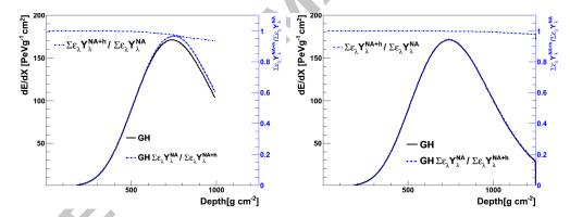
Figure 5: Effect of including the humidity contribution in the profile of energy deposited for  $30^{\circ}$  (left) and  $60^{\circ}$  (right) zenith angles for a Fe shower of  $10^{20}$  eV. Notice that the dependence of the FY ratio with slant depth varies with the incoming angle. See text for details.
