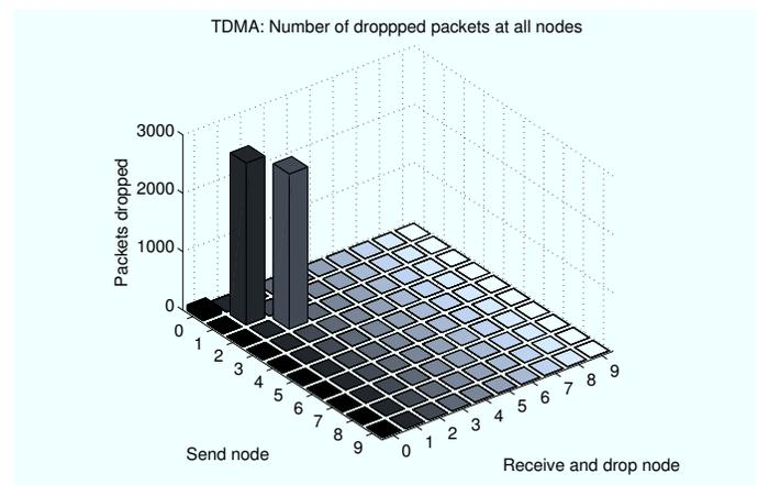
Fig. 3. Packet drop using TDMA. Simulation time = 60 sec.
