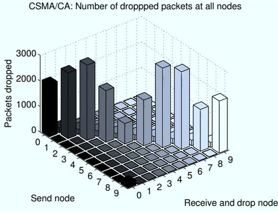
Fig. 4. Packet drop using CSMA/CA. Simulation time = 60 sec.
