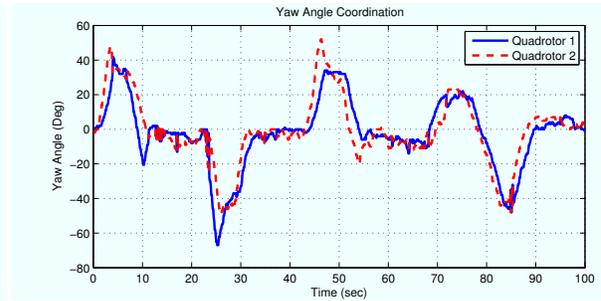
Fig. 12. Average consensus for the yaw subsystem. An external reference was given to the system in order to show the delay over the wireless network
