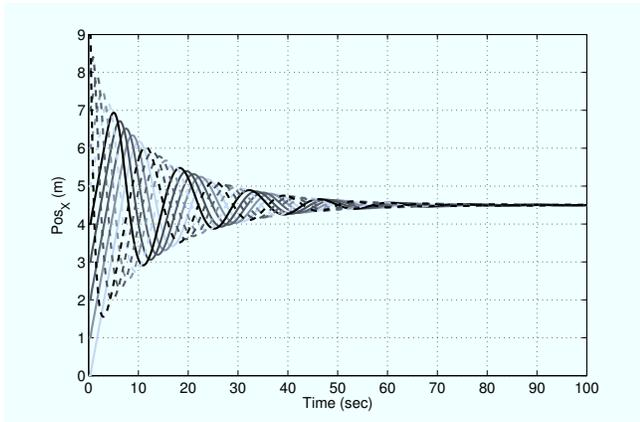
Fig. 6. Multiple quadrotor consensus with  $\tau_{ji} = \tau_{kj}$
