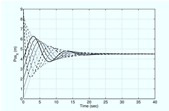
Fig. 2. Multiple quadrotor consensus using perfect communication
