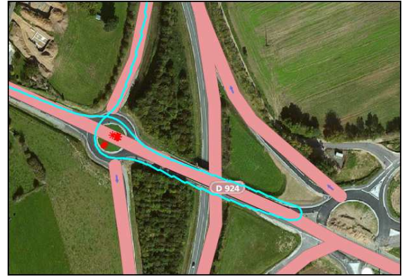
Fig. 6. Example of application of the algorithm in rural environment. Here the road network has changed recently, one roundabout has been created and another one is being built. These are not registered in the digital map (red lines) yet. The vehicle track is in blue and the centres of the roundabouts found by our algorithm are in red stars.
