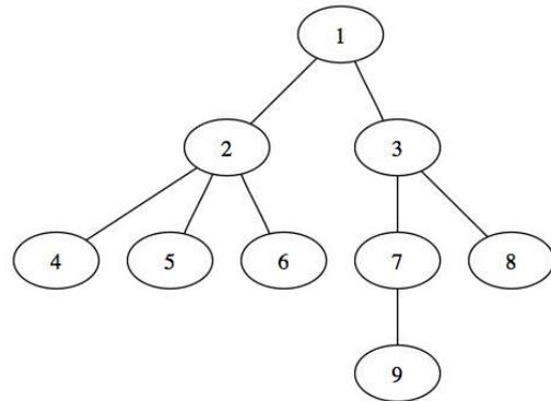
Figure 1. Example of rooted tree with 9 nodes (1-9).
