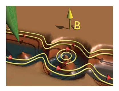
FIG. 1: Artist view of edge states in the quantum ring confining potential. To simplify, we have assumed that no edge state is reflected at the ring's openings, which may not be the case in the real quantum ring. The tip, in green, induces a local perturbation of the potential that can be scanned over the quantum Hall interferometer.
