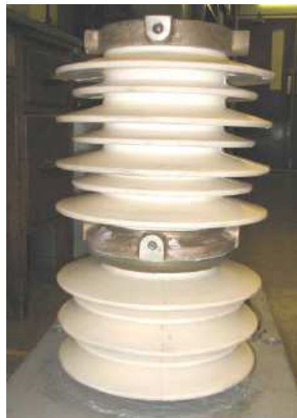
Figure 1. Overall view of the hollow insulator.
