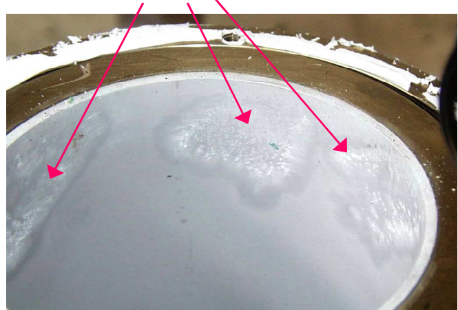
Figure 5. Evidence for HTV liner discoloration on failed insulator
