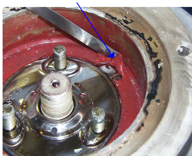
Figure 6. Examination of RTV gasket in failed insulator
