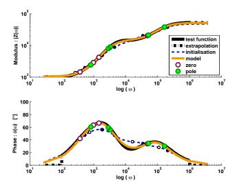
Figure 17: The GMM obtained after the optimization of parameters given by the method described in Section 4.1 (see Table 8 in Appendix C). The optimization is proceed thanks to the method, described in Section 4.2.2, using asymptotes to translate model deviations from the test curves into parameters steps. The optimized parameters are detailed in Table 10 in Appendix D. The indicators of such parameters are  $\delta_{|Z|} = 0.77\%$  and  $\delta_{ig} = 0.15\%$ .
