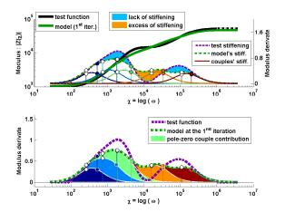
Figure 13: Modulus of the test function and its derivative compared to the model's ones with the couple contributions during the 1st iteration
