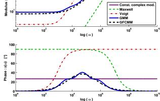
Figure 1: Complex shear stiffness of a multilayer viscoelastic material at ambiant temperature in the [200-3500Hz] frequency range. The top graph represents the normalized modulus H(f)/H(f=200Hz) (dimensionless) and the bottom graph represents the phase  $\psi$  (in degrees).
