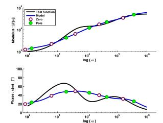
Figure 8: CRONE's graphical method [22]. Pole Zero couples are detailed in Table 5 in Appendix C. The indicators of such parameters are  $\delta_{|Z|}=23.48\%$  and  $\delta_{\varphi}=8.24\%$ .
