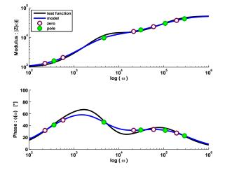
Figure 7: Enclosing Curves Method. Pole Zero couples are detailed in Table 4 in Appendix C. The indicators of such parameters are  $\delta_{|Z|}=4.5\%$  and  $\delta_{\varphi}=1.25\%$
