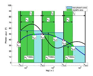
Figure 5: CRONE's graphical method [22]. The areas under the asymptotes curve and under the test curve are equal. The width  $\alpha_i$  give the distance between poles and zeros.
