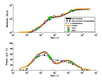
Figure 12: The GMM obtained after the optimization of parameters given by the method described in Section 4.1 (see Table 8 in Appendix C). The optimization is proceed thanks to a Matlab<sup>®</sup> function based on the Nelder-Mead Simplex Method. The optimized parameters are detailed in Table 9 in Appendix D. The indicators of such parameters are  $\delta_{|Z|} = 0.11\%$  and  $\delta_{\varphi} = 0.03\%$ . Notice that the fourth Pole is lower than the fourth Zero, thus it is non-causal.
