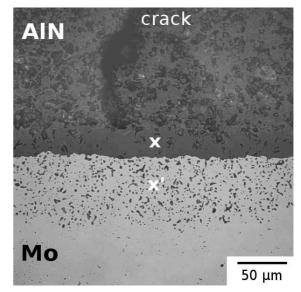
Figure 3. Optocal microscope observation of the cross section of an AlN/Mo assembly. The "X"s indicate zones where EDX measurements were performed to analyze the chemical species present close to the interface
