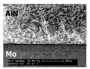
Figure 2. Cross-sectional SEM photo of Mo/AlN interface
