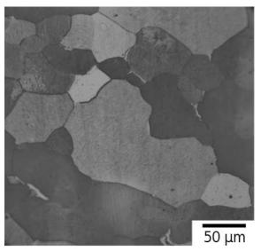
Figure 1. Cross-sectional optical micrograph of bulk molybdenum
